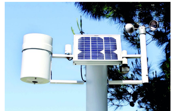
Several weather stations monitor campus microclimates for irrigation control. Image: RainMaster.
